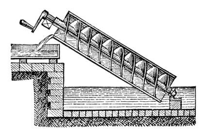
The Archimedes' screw, Archimedean screw, or screwpump is a machine historically used for transferring water from a low-lying body of water into irrigation ditches. It was one of several inventions and discoveries traditionally attributed to Archimedes in the 3rd century BC.
